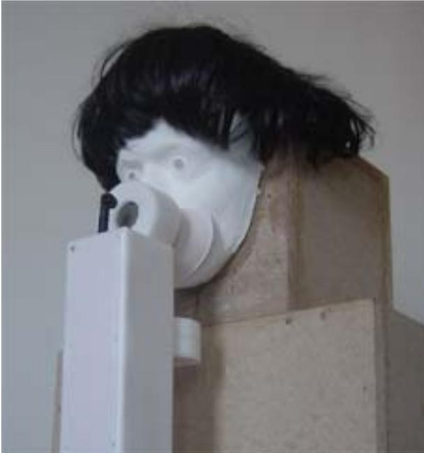
**Fig 4** Artificial head loudspeaker to study acoustic distortion
